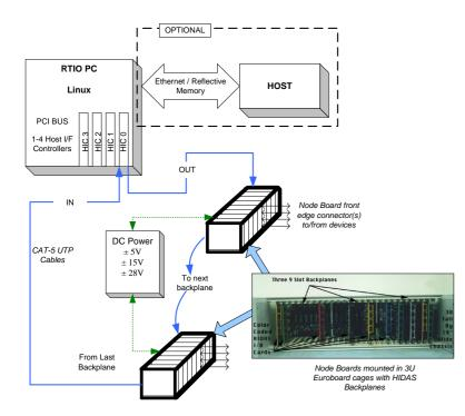
Messages originate from software and are transmitted to the first node board in the ring via the HIC.
